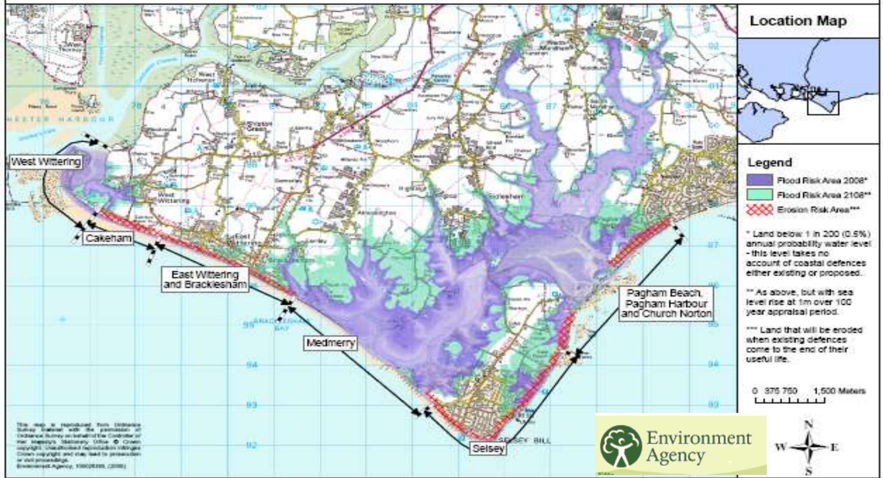
Figure 1.2 - Strategy extent with flood and erosion risk
