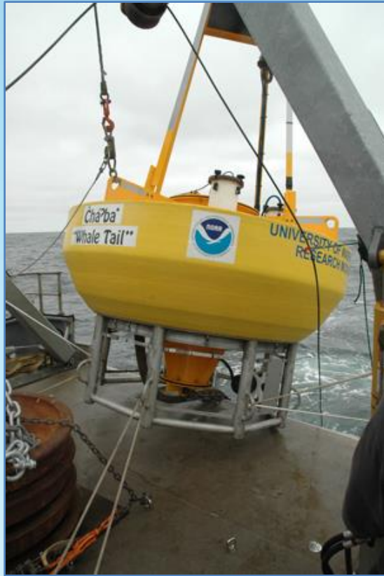
Seawater Monitoring Buoy
