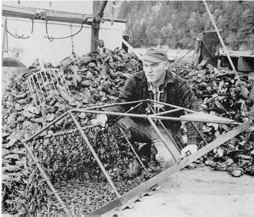
Dick Steele, a partner in the Rock Point Oyster Company, displays a drag dredge. It is towed on the bottom at this angle and slides under the oysters on bottom and into the chain bag, to finally lifted and dumped on deck.
