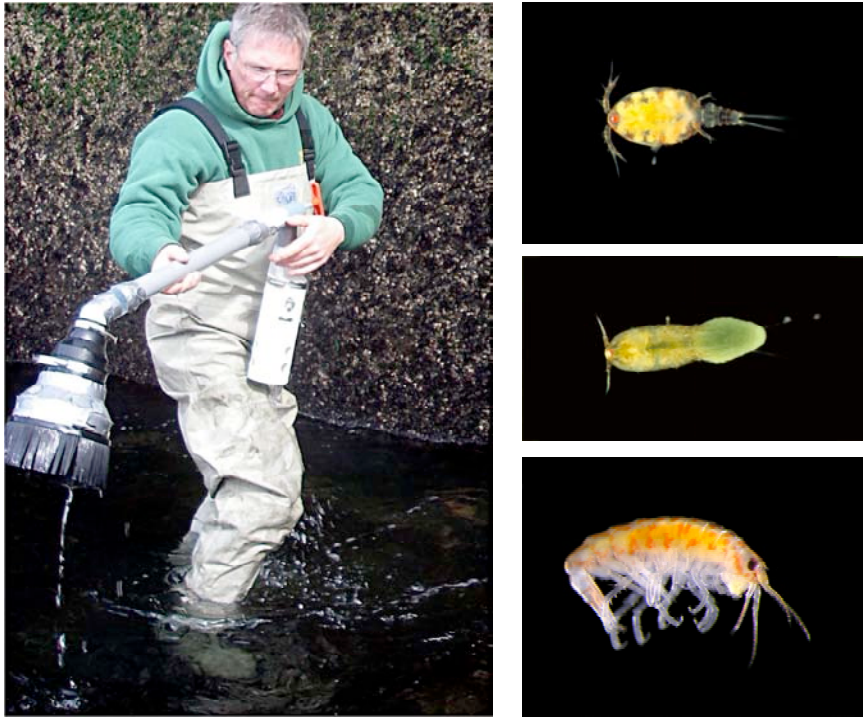
Figure 4. Left, epibenthic pump used for sampling invertebrates on habitat panels. Right, prominent salmon prey taxa associated with habitat panels: harpacticoid copepods (top), gammarid amphipod (bottom) (not to scale).
