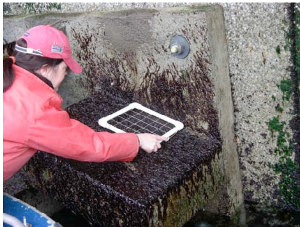
Figure 3. Quadrat sampling algae and sessile invertebrates on seawall test panel.
