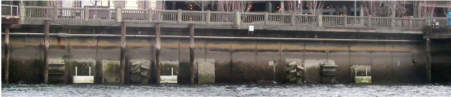
Figure 2. Random placement of experimental habitat panels along Seattle seawall. Light colored objects are troughs containing sediment of three different grain sizes.
