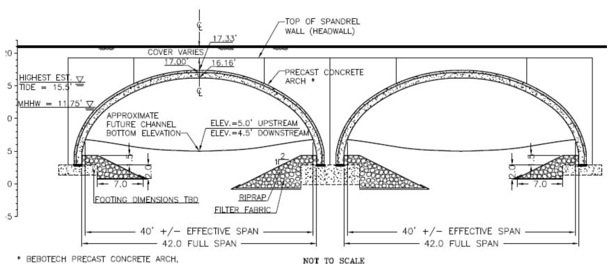
\* BEBOTECH PRECAST CONCRETE ARCH, TYPE E36/4. MINIMUM EFFECTIVE SPAN = 40'. MUST PASS MHHW = 11.75'. MUST MAINTAIN TOP OF FOOTING @ ELEV = -3.0'
