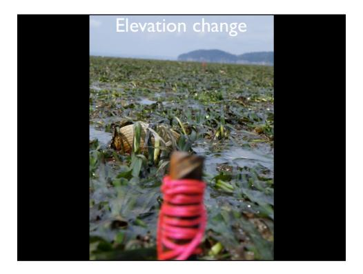
We measured changes in elevation by installing rebar stakes at 8m intervals on a line perpendicular to the farm boundary. By stringing mason line taut across the top of two rebar stakes, we measured the distance from the line to the sediment surface at set intervals, and collected data before and after each aquaculture event, in and outside of the farmed zone.
