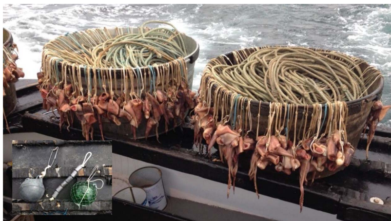
Fig. 2. Floated demersal longline tub gear, staged on the stern of the vessel in preparation for setting. Inset photo shows two styles of floats (hard plastic and glass) with a typical 20 oz. (567 g) weight placed in between the floats. The floats and weights were coiled within the tubs when gear was prepared for setting.
