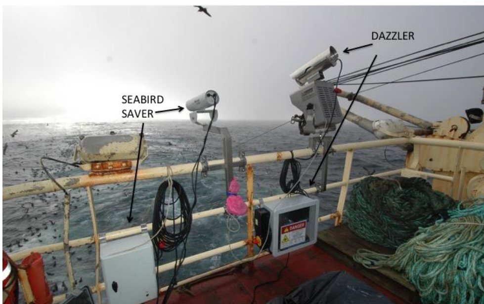
Figure 2. SeaBird Saver (left) and Dazzler (right) lasers mounted on the stern of a Pacific hake trawl catcher processor.
