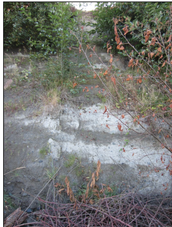
Figure 7. Exposure directly north of the assessment property where the bulkhead has caused end-effect erosion. Lower bluff sediments are mapped as undifferentiated non-glacial silt, sand, and gravel. Bluff height at this location is about 25-30 ft.
