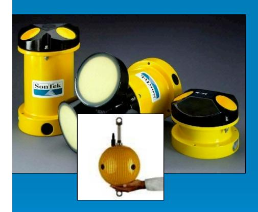
ADCPs and S4 Current Meter (courtesy of SonTek/YSI, Inc. and Interocean Systems, Inc.)
