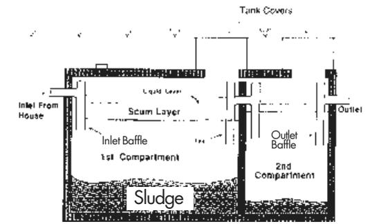
8) **Baffle condition.** Baffles direct septic flow and help prevent sludge and scum from traveling into the drainfield area. The pumper should make sure the baffles are intact and functioning. In a two-compartment tank there are three baffles that should be examined: the inlet, center, and outlet. In a single-compartment tank the center baffle would not exist. Baffles can be repaired or replaced easily by your pumper.
